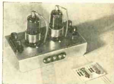
Photo A—Amplifier in standard and in printed form. Photo B, below — The same two amplifiers, bottom view.
